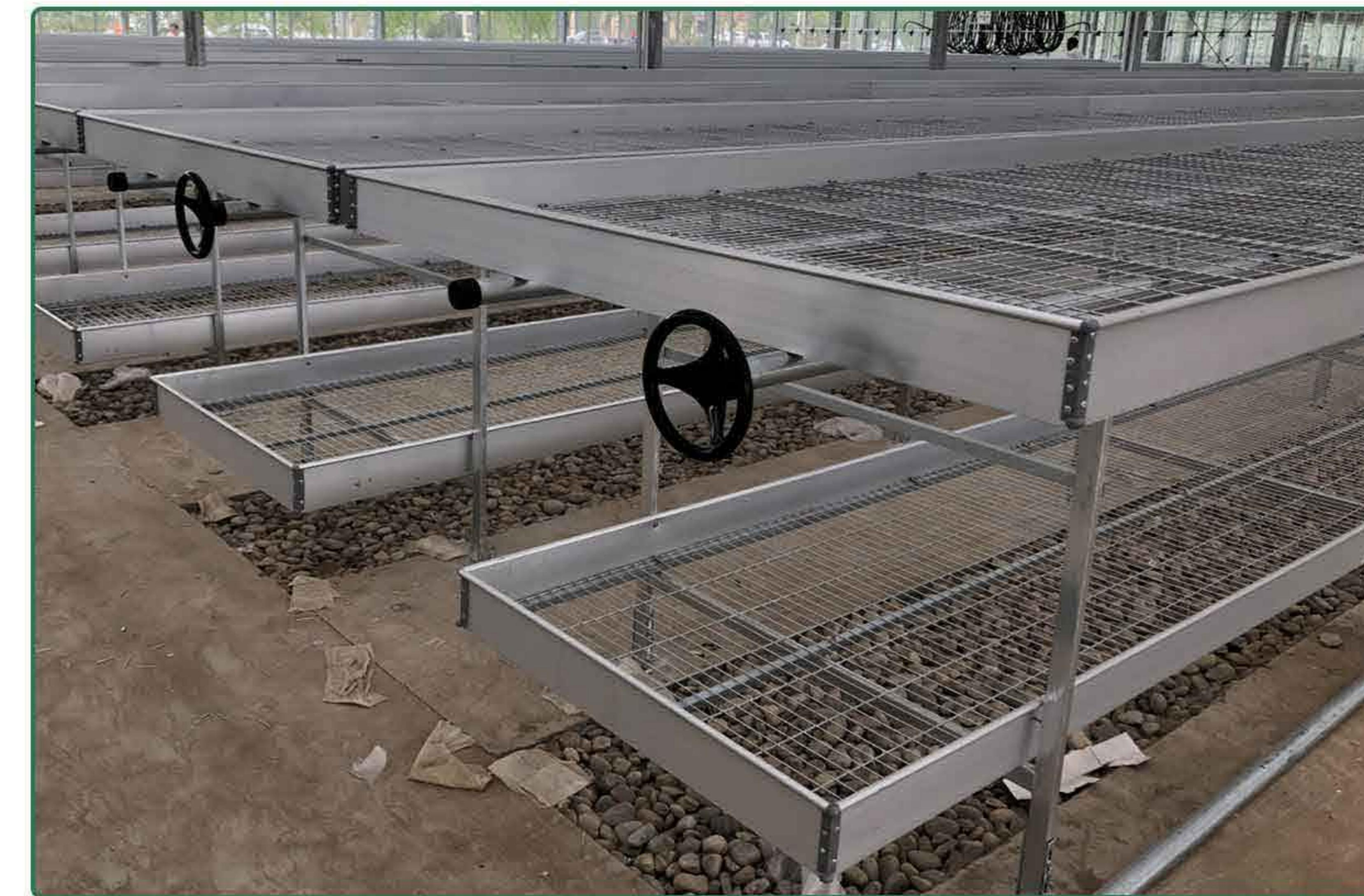
The seedbed support is made of hot-dip galvanized steel pipe, the frame is made of aluminum alloy, and the surface of the seedbed net is treated with anti-corrosion coating; Height can be fine-tuned, with anti-roll limit device, and can produce 0.8m action between any seedbed industry channel.
